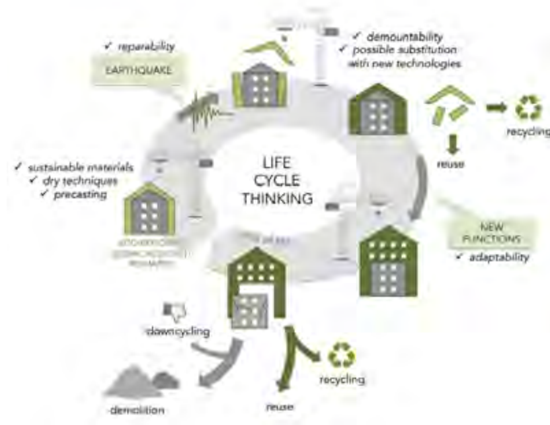
Figure 130: Diagram to illustrate the life cycle thinking for recycling materials and buildings. (Source: https://www.researchgate.net/publication/319464500_Combining_seismic_retrofit_with_energy_refurbishment_for_the_sustainable_renovation_of_RC_buildings_a_proof_of_concept )
