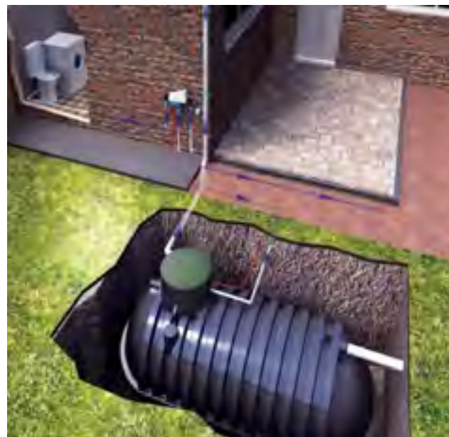
Figure 97: Example of an underground water tank in relationship with the building (Source: https://handymantips.org/about-underground-water-tanks/ )
