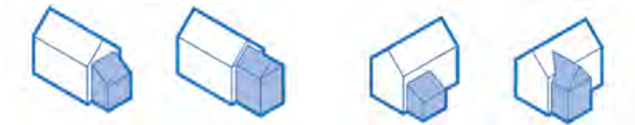
Figure 122: Good examples for side extensions, respecting existing building scale, massing and building line.
