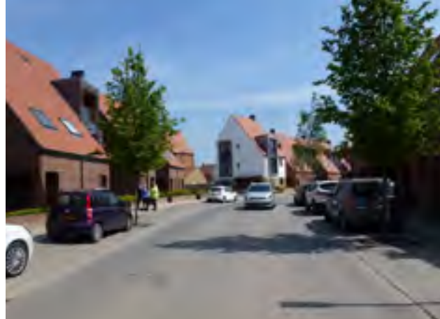
Figure 67: Secondary street with inset parking bays alternating with street trees on both sides of the street in Derwenthorpe, York.
