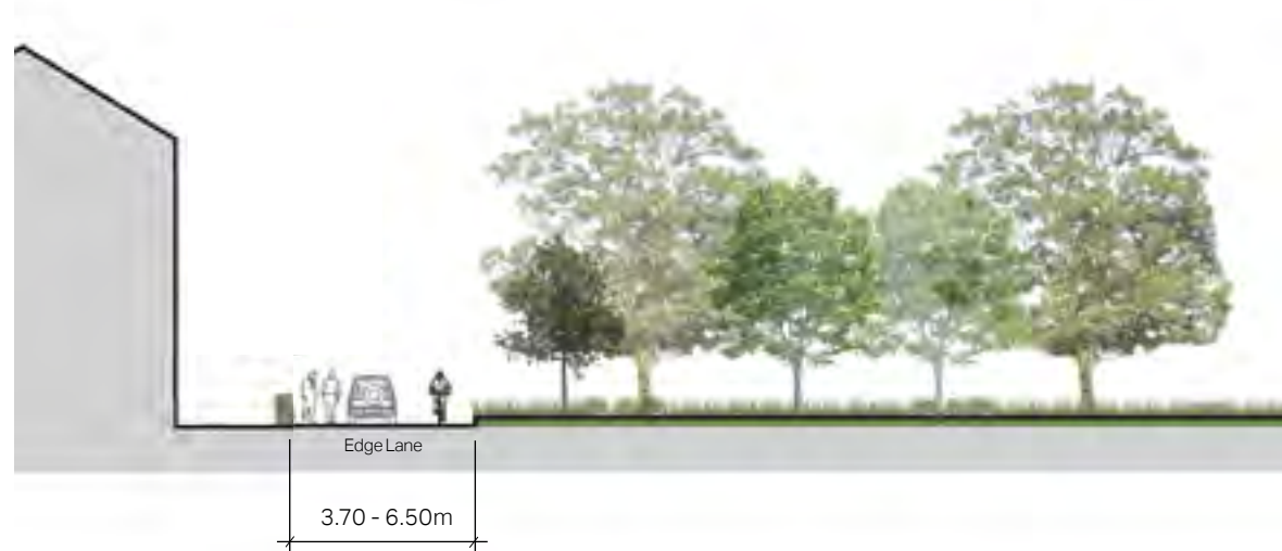
Figure 64: Cross-section to illustrate some dimensions for edge lanes.
